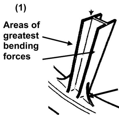
The forces are concentrated at the outer edges of the beam (1) thus this is where the largest amount of material needs to be located. (1)
